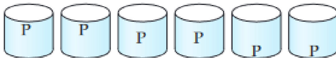
(g) RAID 6: P+Q redundancy
