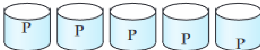
(f) RAID 5: block-interleaved distributed parity
